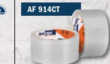
Linered cold temperature aluminum foil tape for joining and sealing aluminum-backed and fibrous insulation and metal ductwork, and can also be used in the industry to repair metal and sheet metal that may have been damaged by water or fire. Designed with an acrylic adhesive and tested in accordance with UL 723, AF 914CT delivers an airtight seal in temperatures ranging from -20 F to 260 F.
